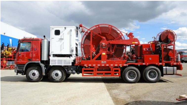
NOV – Coiled tubing unit
