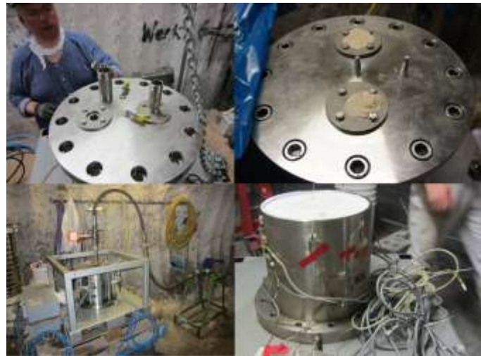
Fig. 14: Device for measuring the development of swelling pressure and temperature during hardening of Sorel concrete A1.
