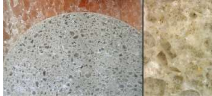
Fig. 2. Sorel concrete A1 embedded on the left in reddish rock salt. The maximum grain size of the concrete is about 4 mm. The grains of the aggregate are the irregular, dark areas in the light gray matrix. On the right is a microscope photo that shows the concrete at a higher magnification.
