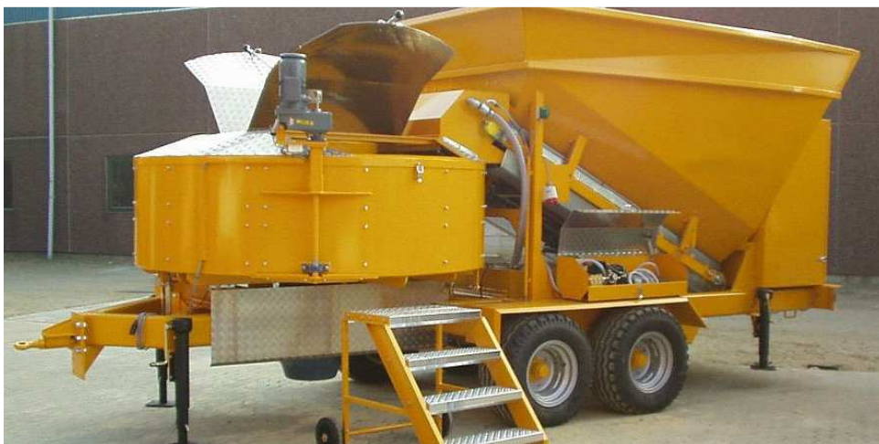
Fig. 6: Mobile mix plant assembled on a joint twin-axle bogie trailer.
