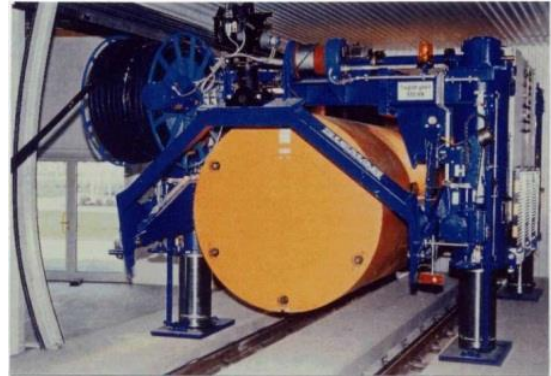
Fig. 8. Test facility for drift disposal of spent fuel canisters (POLLUX ® -10) (11)
