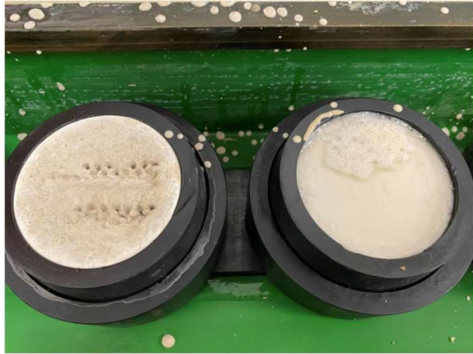
Figure 8 – left: Sorel concrete with anhydrite powder (8%); right: without anhydrite powder.
