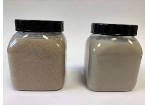
Figure 9 – left: Sorel concrete without anhydrite powder; right: with anhydrite powder.
