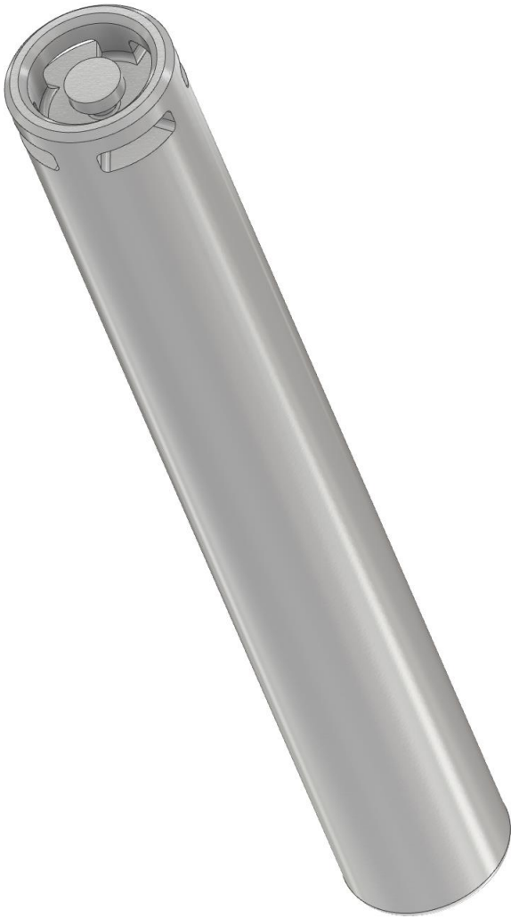
Figure 2: Isometric view of the canister with showing the hook area.
