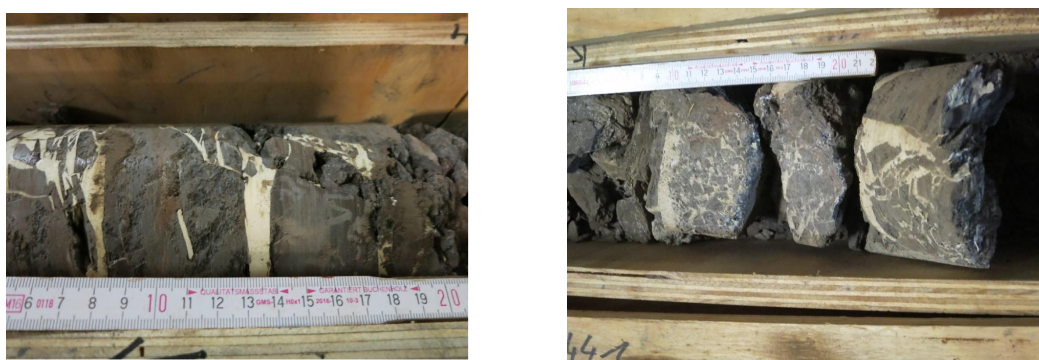
Figure 2. Core samples from pilot tests – claystone (gray) and injection grout (ochery)
