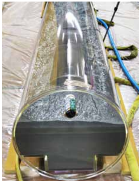
Mock-up test demonstrating the feasibility of a void free backfilling of the disposal drifts
