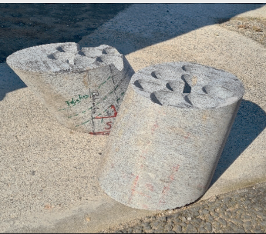
Drill cores of Freiberg gneiss used as samples for laboratory tests to determine the rock properties (R&D project BARIK)
