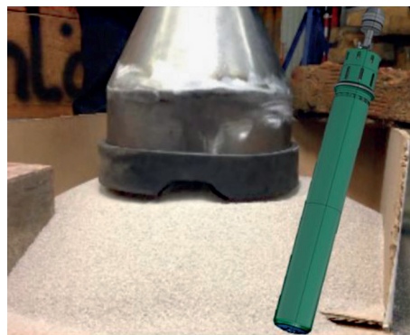
Demonstration test with a suction bell for the removal of backfill material from a disposal borehole
