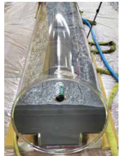
Mock-up test at a scale of 1:6 to demonstrate the feasibility of backfilling disposal galleries without residual voids
