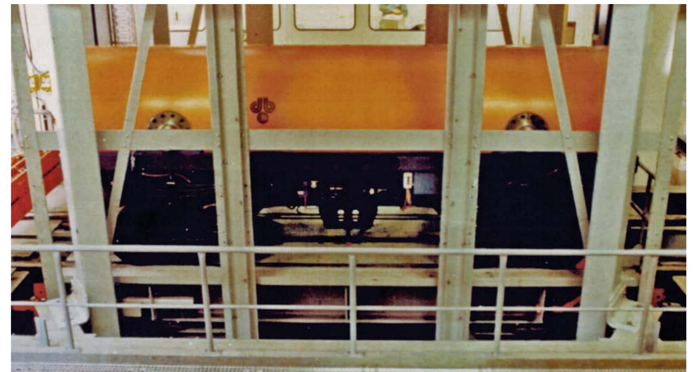
Demonstration test for the shaft transport of waste containers
