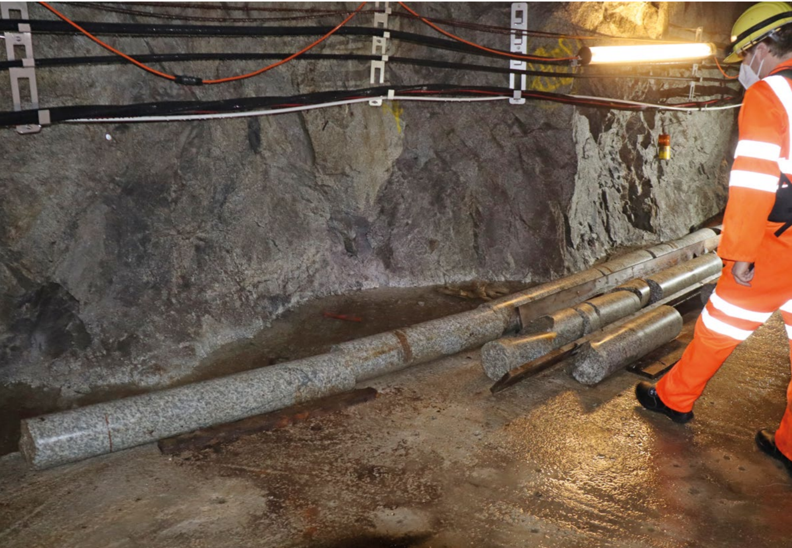
Drill cores from exploration work in the Bedretto underground laboratory (Switzerland)
