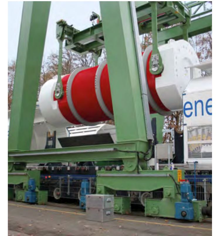
Reloading of a CASTOR® cask (Source: GNS)
