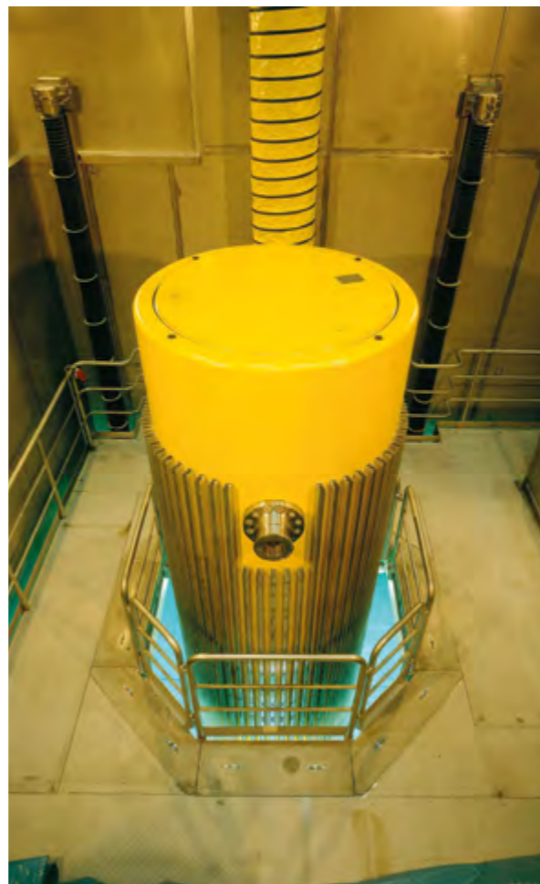
POLLUX® cask at the maintenance point of the pilot conditioning plant in Gorleben (Source: GNS)
