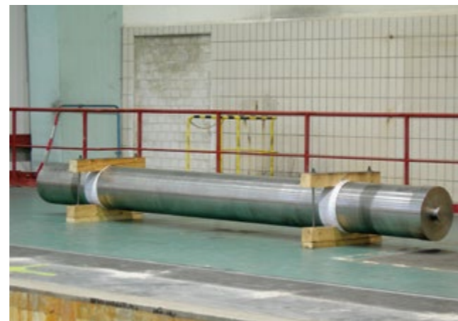
Mock-up of a spent fuel canister
