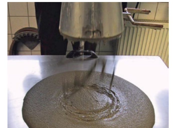
Settlement test to assess the consistency of fresh concrete
