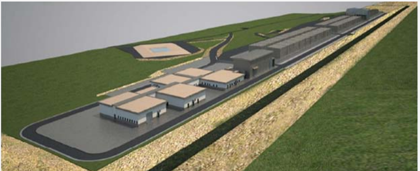
Diagram of the National Disposal Facility for low and intermediate level waste at Kozloduy, Bulgaria (Source: SERAW)
