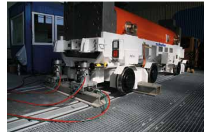
Remedial action of an operational disturbance: demonstration of re-railing a derailed transport cart with transfer cask
