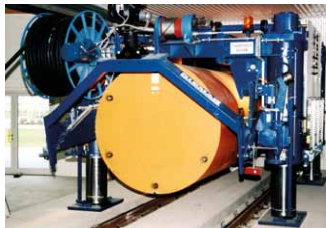
Demonstration test for the emplacement of POLLUX® casks containing the fuel rods of spent fuel elements
