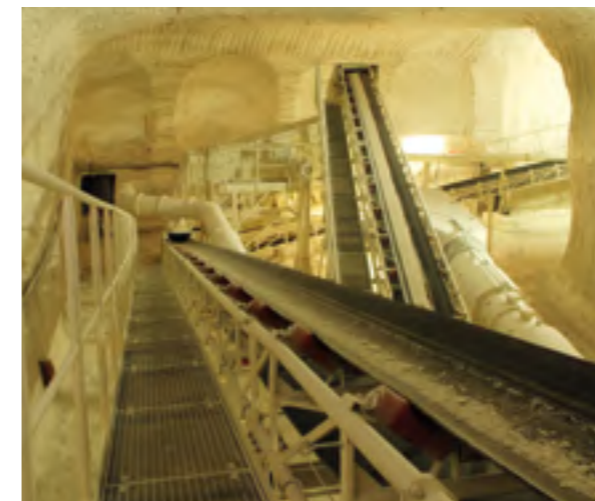
Part of the salt processing plant for the production of sorel concrete
