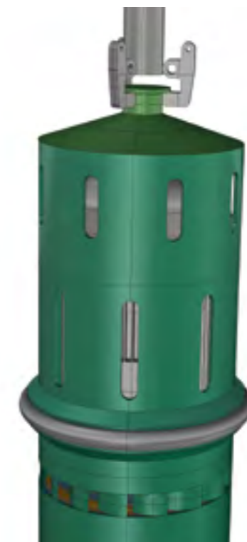
Concept of a suction bell (top section) to remove loose backfill material from an emplacement borehole
