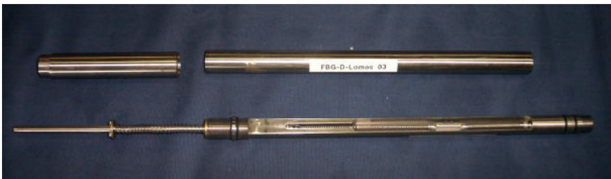
Fig. 3.5: Photo of the interior of the displacement cell FBG-D-Lomos 03 .
