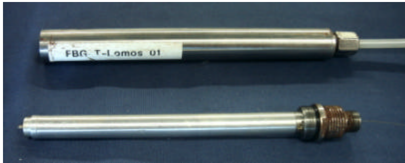
Fig. 3.6: Photo of the interior of a temperature sensor used in Konrad
