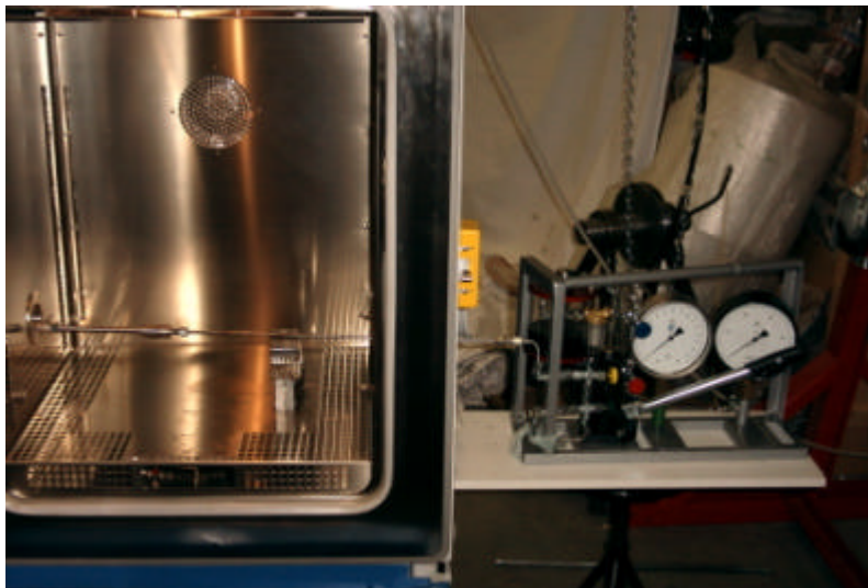
Fig. 1.27: Calibration set-up, pore water pressure sensor
