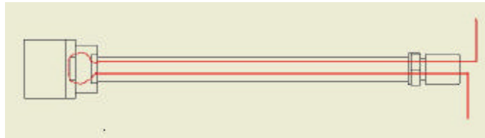
Fig. 1.38: Fibre path for establishing series configuration.
