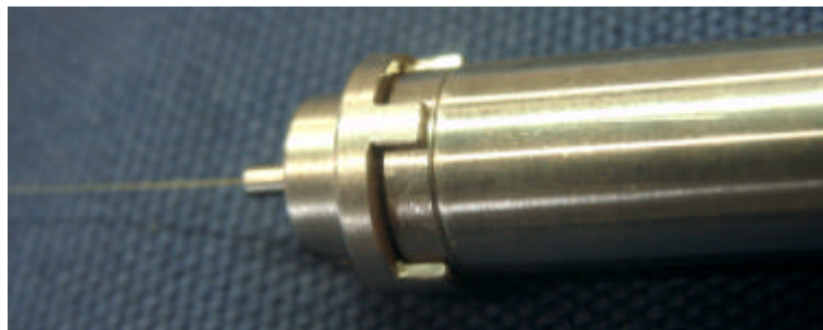
Fig. 3.8: Zoom of the interior of the water leakage sensor FBG-WL-Lomos 01
