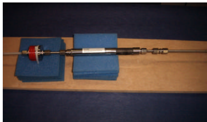
Fig. 3.20: End sensing line riser cap.
