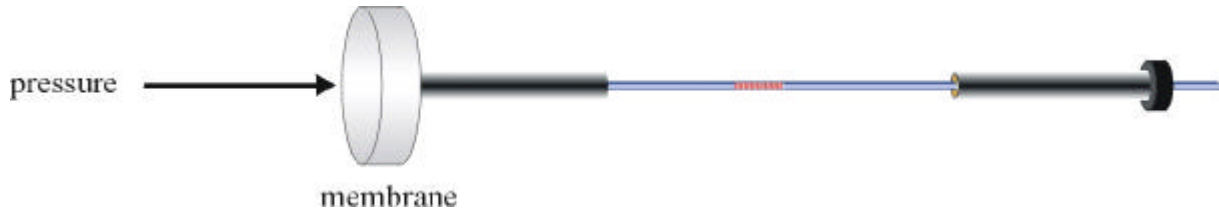
Fig. 1.18: Basic design of the membrane pressure sensor
