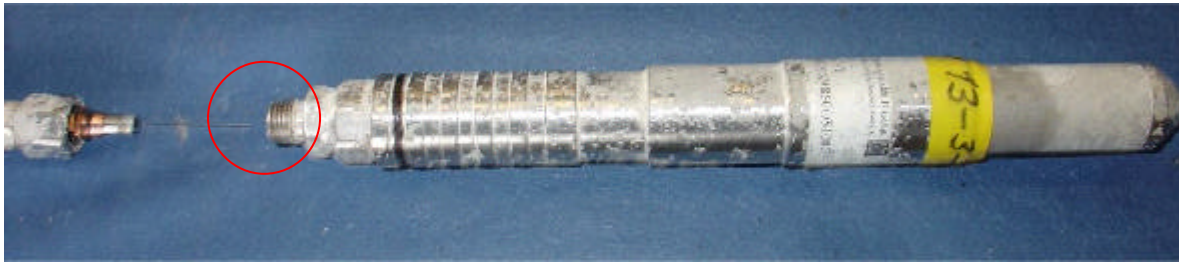
Fig. 3.34 MPWP FOS broken at temperature grating
