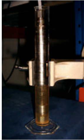
Fig. 1.45: Test set-up water leakage sensor in salt solution.
