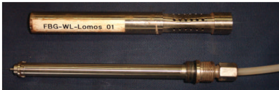
Fig. 3.7: Photo of the interior of the water leakage sensor FBG-WL-Lomos 01
