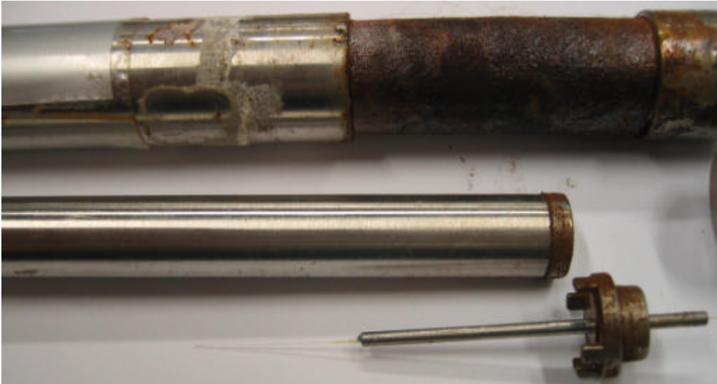
Fig. 3.52 : Photo of inner components of the damaged water leakage sensor SN01102504.
