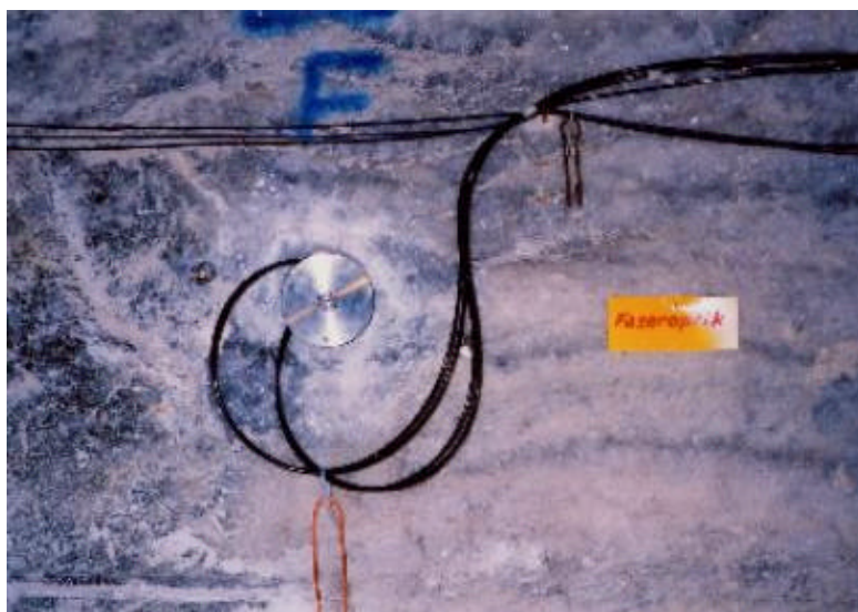
Fig. 4.14: Front plate of the installed strain cable with out coming fibers for deformation and temperature measurements
