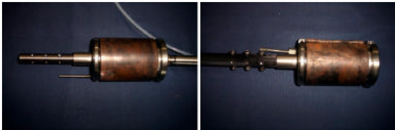
Fig. 4.13: Carbon - Packer fixation mechanism
