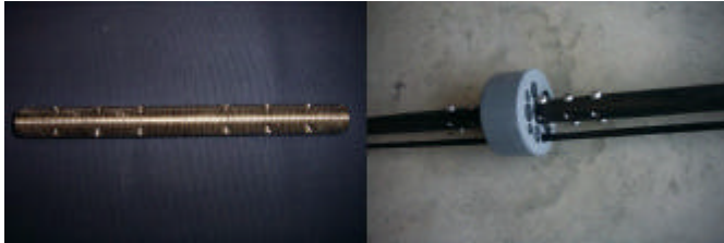
Fig. 4.12: Connection piece for carbon rods and dummy packer
