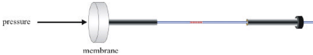
Fig. 4.17: Basic design of the membrane pressure sensor
