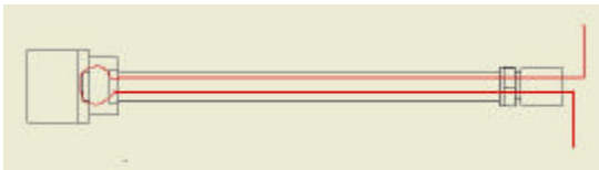
Fig. 4.22: Fibre path for establishing series configuration.
