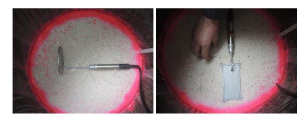
**Fig. 3.26** Two hydraulic pressure cushions were installed in the lower third of the filled cell while filling it with the crushed salt material. One records the horizontal, the other records the vertical acting pressure
