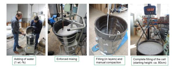
**Fig. 3.14** Preparation of the "large IfG oedometer cell": Salzgrus (initial state as delivered, pre-treatment (homogenization) and stepwise filling and weight control of the cell
