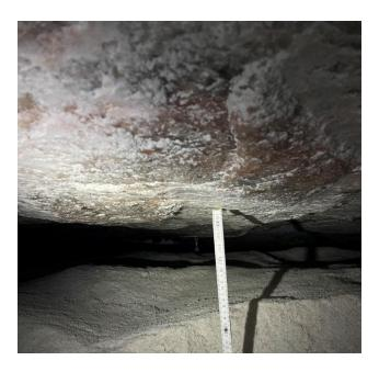
**Fig. 2.15** Measurement of gap between the KOMPASS backfill body and the roof of the drift /SCH 23/
