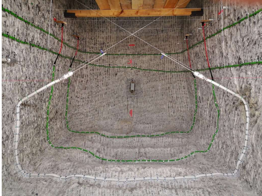
Figure 3 - Installed test chamber 3 (white hose).
